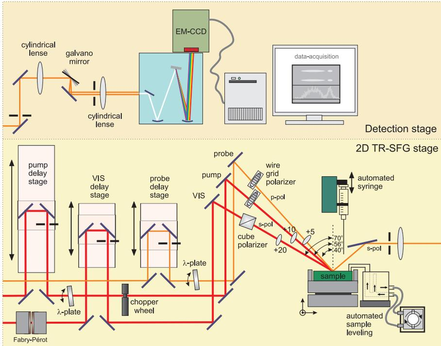
FIGURE 3.4. Schematic representation of the 2D TR-SFG setup.
